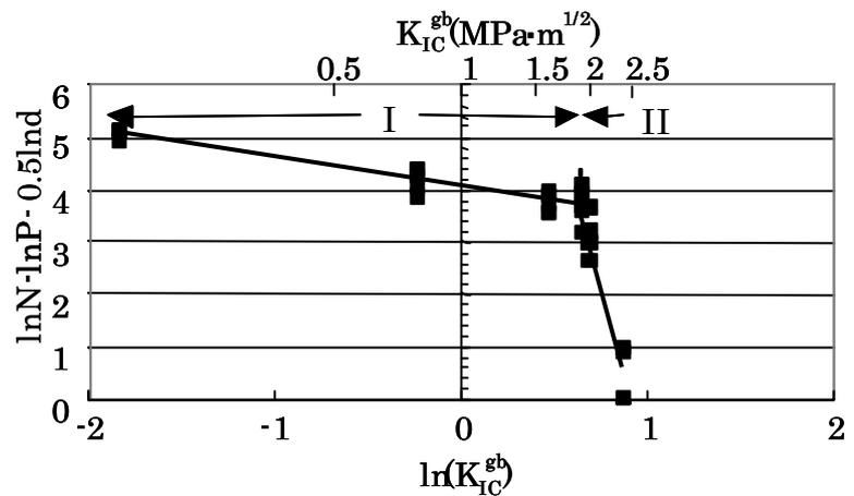
Fig.2 The relationship between the normalized density of microcracks and grain boundary fracture toughness.
