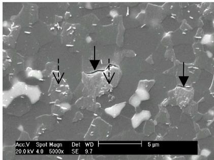
Fig.1 A typical SEM image of the sliding tested AlN surface. Solid arrows indicate grain boundary microcracks and broken ones indicate silicon debris.
